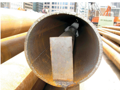
Figure 3. Custom welded inclinometer base.
